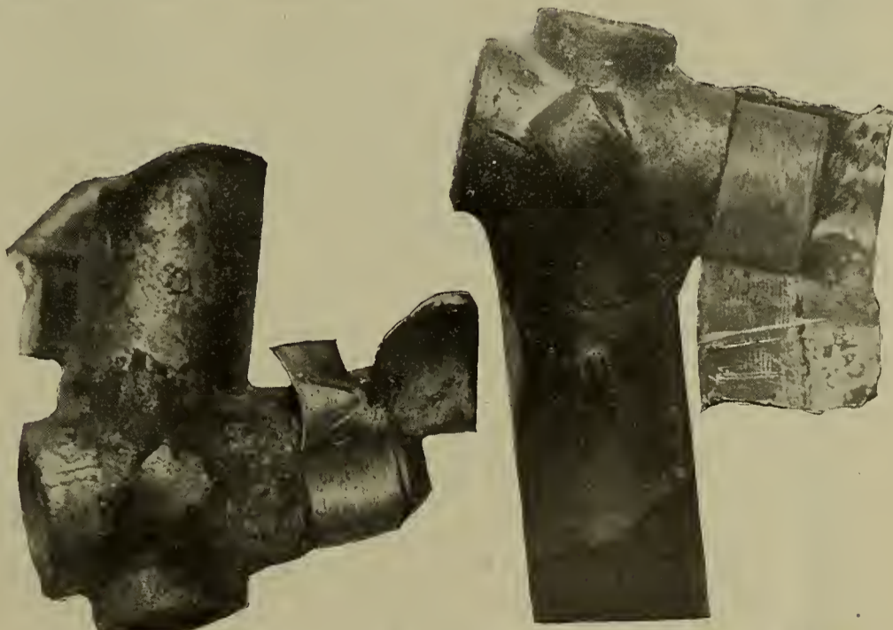
Results—The piece to the Right was Brazed by Dipping; that on the Left was Brazed by Flame.
